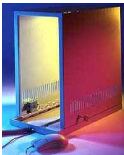
Mouse and keyboard cable entrapment
